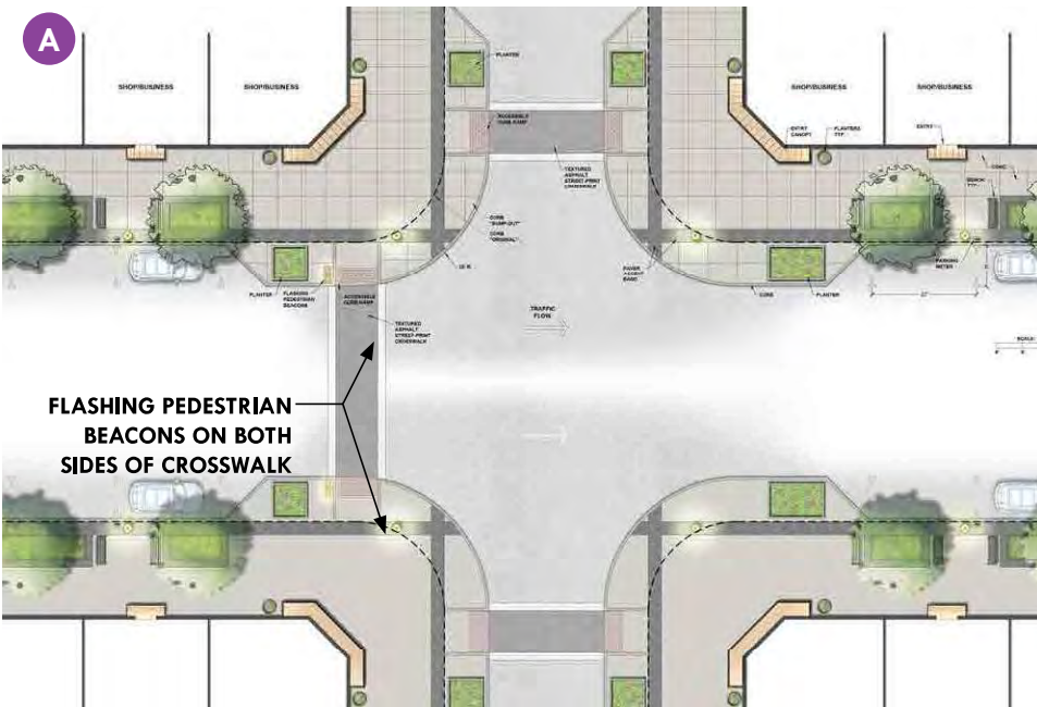
Plan view design of a typical Main St. intersection showing flashing beacons, textured crosswalks on the north side, bluestone accent bands, street trees and planters.
