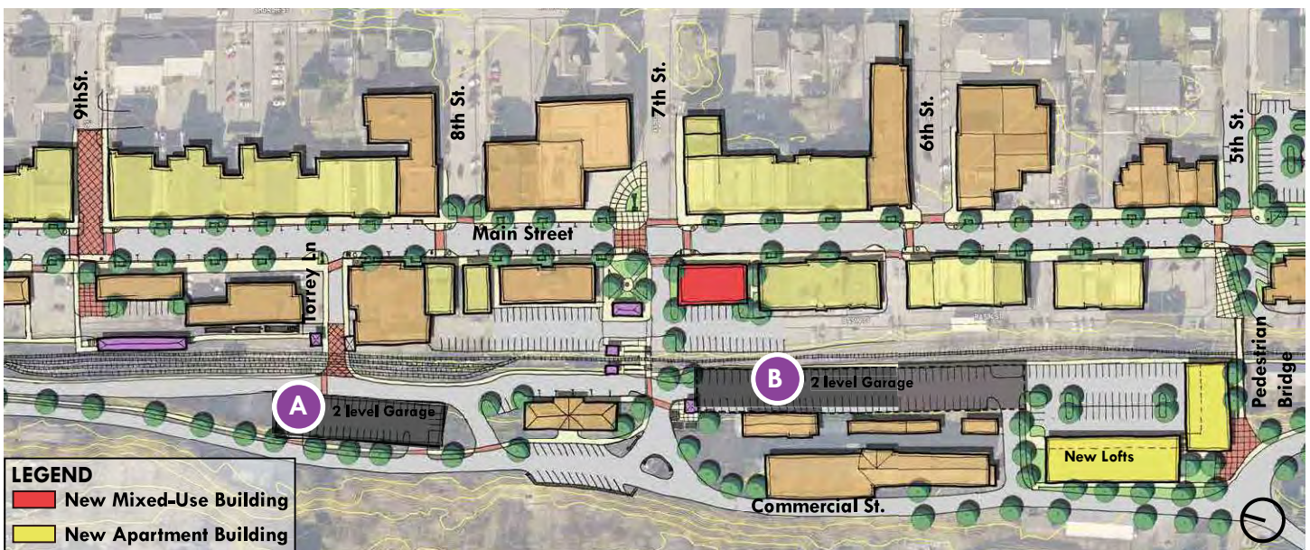
Proposed plan view of potential parking improvements featuring (2) 2 level parking decks along the railroad tracks.
