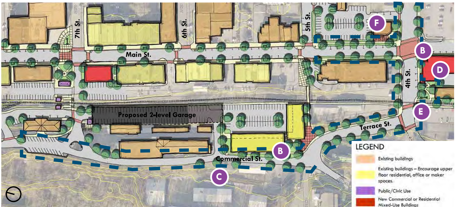
Plan view of proposed Commercial St. Gateway improvements including adding new sidewalks, lighting and street trees along commercial street with a potential new mixed use building.
